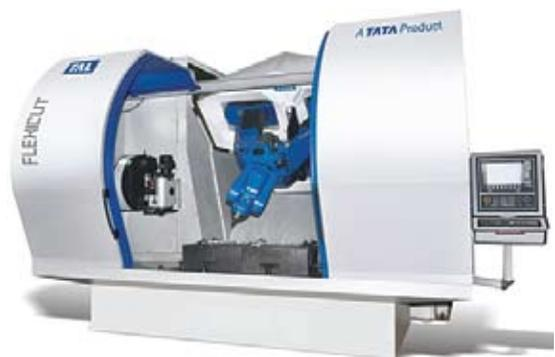
Flexicut-multi axis simultaneous machining operating on parallel kinematics
